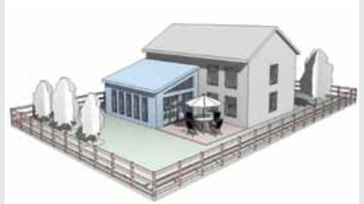
A typical example of a single-storey rear extension in ROI, 40 m 2 or less, that can be added to a detached home without requiring Planning Permission. There are several ways your home can be altered or extended without requiring Planning Permission.
